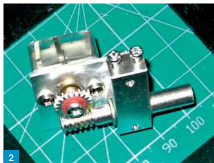
Fig. 1: Circuit diagram. Fig. 2: The polyvaricon capacitor. Fig. 3: The polyvaricon fitted to the circuit under test. Fig. 4: The PCB (not to scale). Fig. 5: Layout of the author's prototype.
